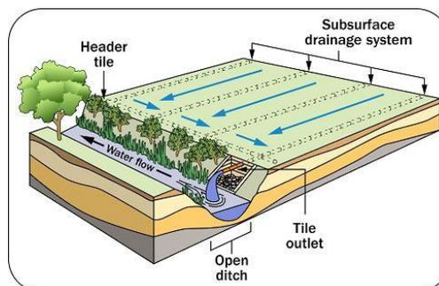
tracks. It is important to maintain relatively smooth, level ground for orchard work and harvesting. Tile drainage spaced between the rows, and not under where the trees will be planted, will drain excess water from the orchard. Tile contractors can be a year behind in getting to your job, so planning ahead is essential. It also helps to order trees a year or more in advance for large plantings.
